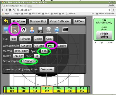
• Enter Microphone Width and Height values. This is the distance measured between the left side of the upper or lower mics, and distance measured between
